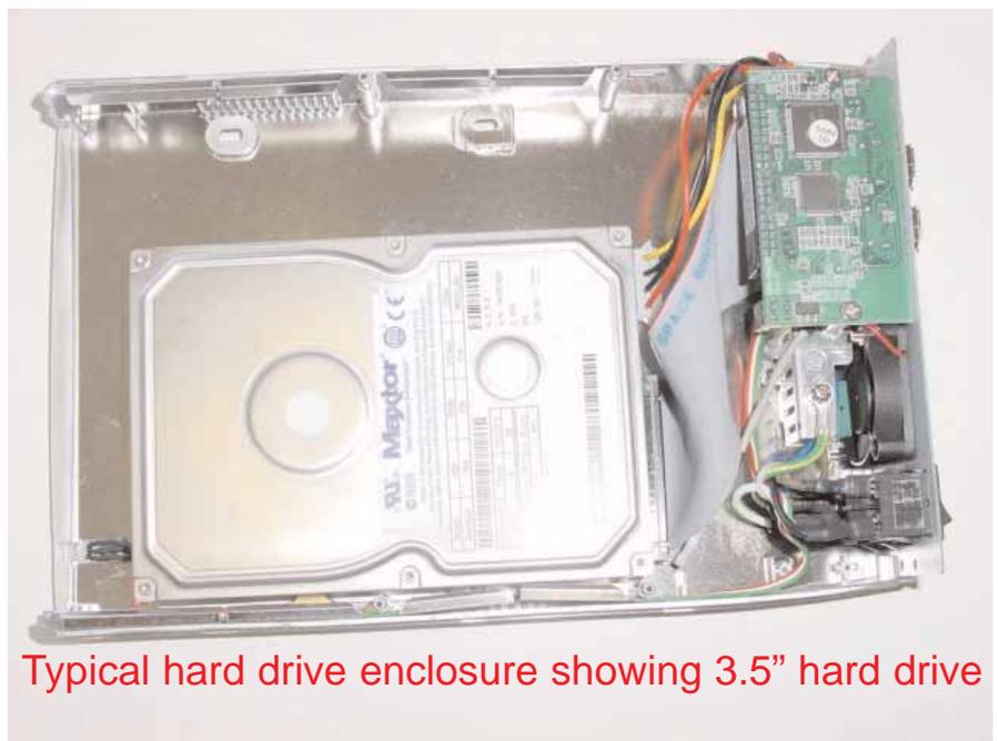
Typical hard drive enclosure showing 3.5" hard drive
