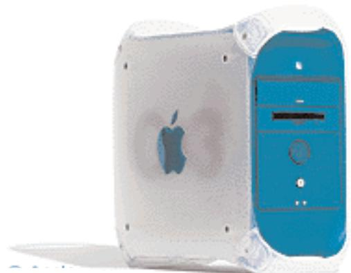
Except for the 300 MHz model, all of the B&W G3 models have a 1 MB backside cache running at half CPU speed. As already noted, this machine was built for throughput.
